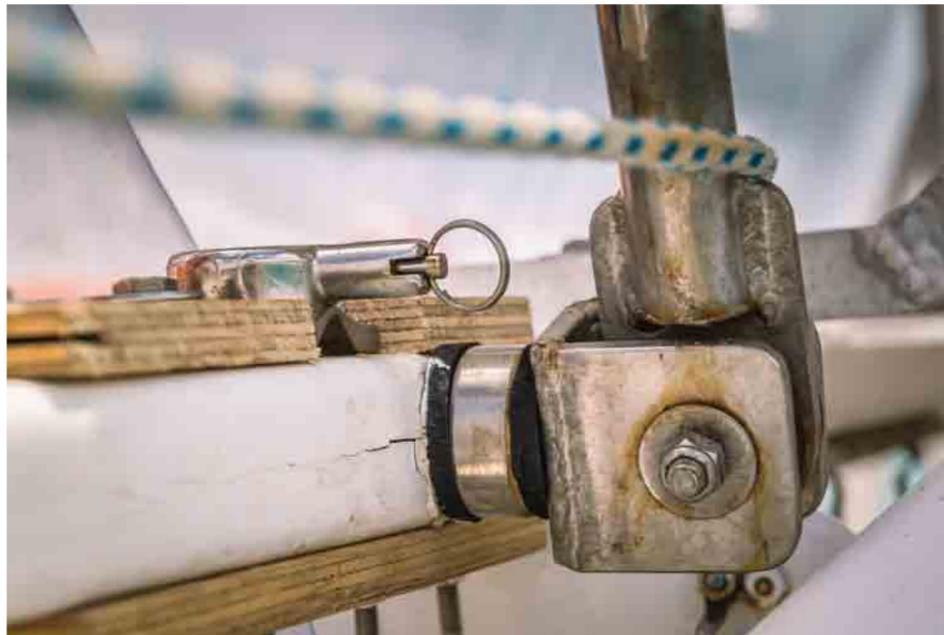
THERE WAS A NASTY CRACK ALONG THE FRAME WHERE THE STRUTS ATTACH... NOT TO MENTION THE DINGHY DAVITS AND THE SOLAR CELLS!
